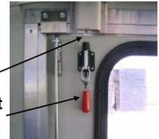
**Shift Interlock System:** If the rear emergency door interlock switch is activated and the bus is started the micro switch sends a signal to the transmission that will not allow the bus to shift into gear. There will also be an audible alarm sounding and the light will illuminate to alert the driver of the situation. The interlock releases when you pull the slide bolt down.
